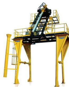
**"DENGAN TEKNOLOGI CORE SAMPLER BERAPA NILAI RENDEMEN BISA DIKETAHUI DENGAN CEPAT. CORE SAMPLER AKAN MENGAMBIL SAMPLE NIRA DARI ATAS TRUK DAN LANGSUNG DIANALISA DI LABORATORIUM CORE SAMPLER. HASIL RENDEMENNYA AKAN KELUAR DALAM WAKTU LIMA MENIT SAJA,"**
